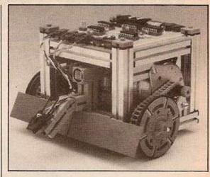
the computerised warehouse. It would use the BCR to follow a line to a set of pigeon holes, then locate a pigeon hole which had been lit up, remove an item with a grab-arm, read its bar codes and use the information given to docket it elsewhere.
